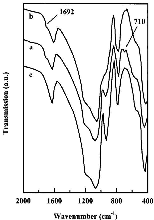
Fig. 3. Infrared spectra of benzoic acid-doped gel glass heat-treated at 200°C (a) and 500°C (b) for 24 hr and un-doped silica gel glass without heat treatment (c).
